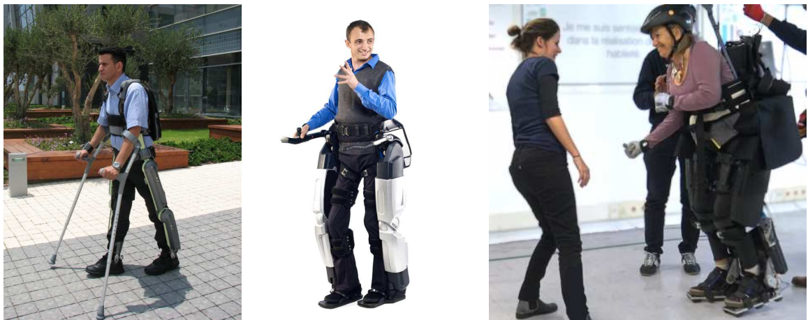
Figure 1 : Left: 4 DoF exoskeleton from Rewalk Robotic. Middle: 10 DoF exoskeleton from Rex Bionics. Right: exoskeleton Atalante from Wandercraft
